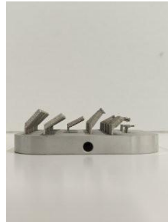
Figure 14. Geometries used in DoE_01 to study the surface roughness of the upskin and downskin surfaces as a function of the build angle.
