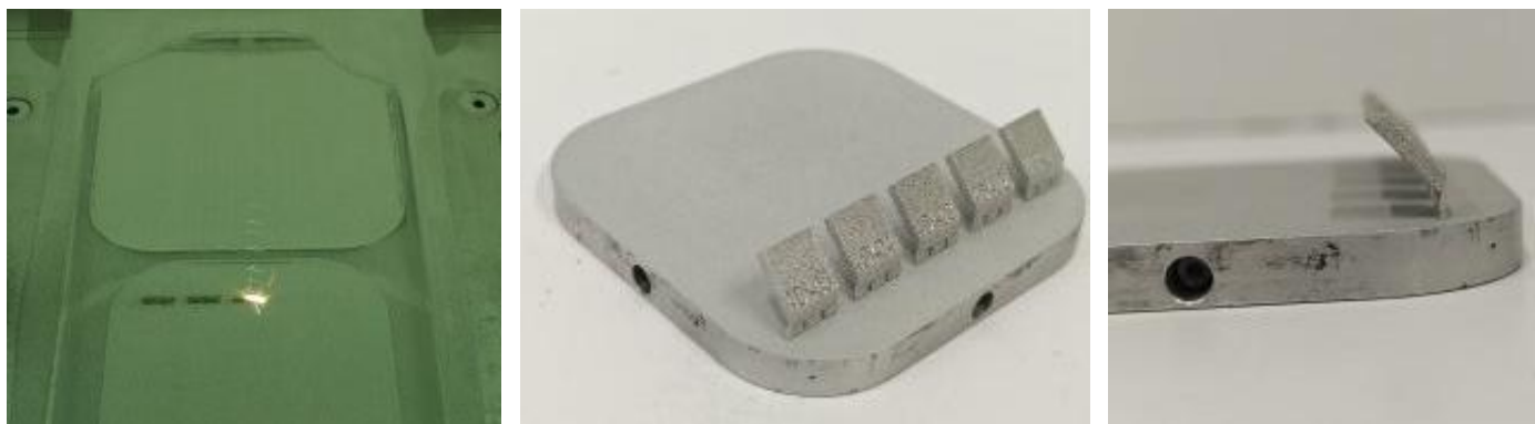
Figure 19. LPBF manufacturing of the material 4 samples used in DoE_02 for the study of the Downskin parameters.
