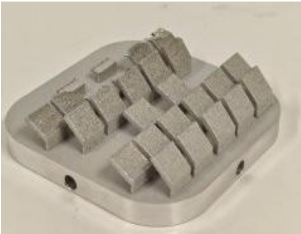
Figure 14. Geometries used in DoE_01 to study the surface roughness of the upskin and downskin surfaces as a function of the build angle.
